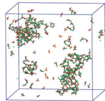
FIG. 2: Representation of (a) unrelaxed and (b) relaxed cubic CdS nanoparticles.
