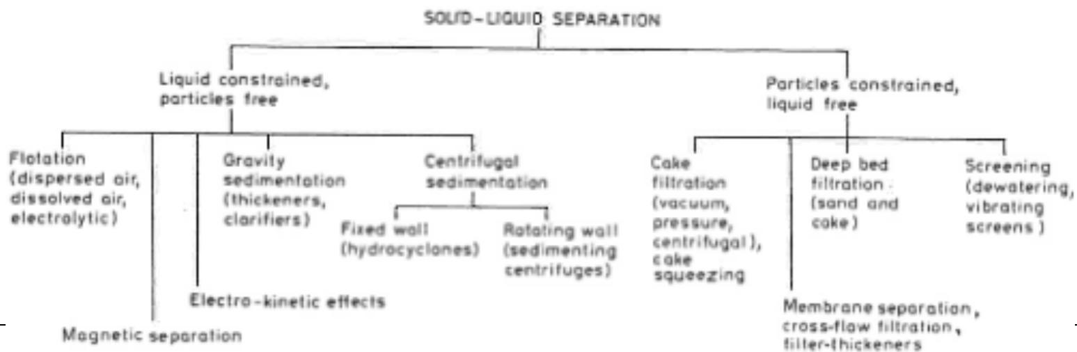
Figure 1.2. Classification of solid-liquid separation processes
